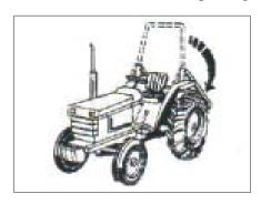
Enclosed cab\_controlled environment-controls climate, comfort and noise
